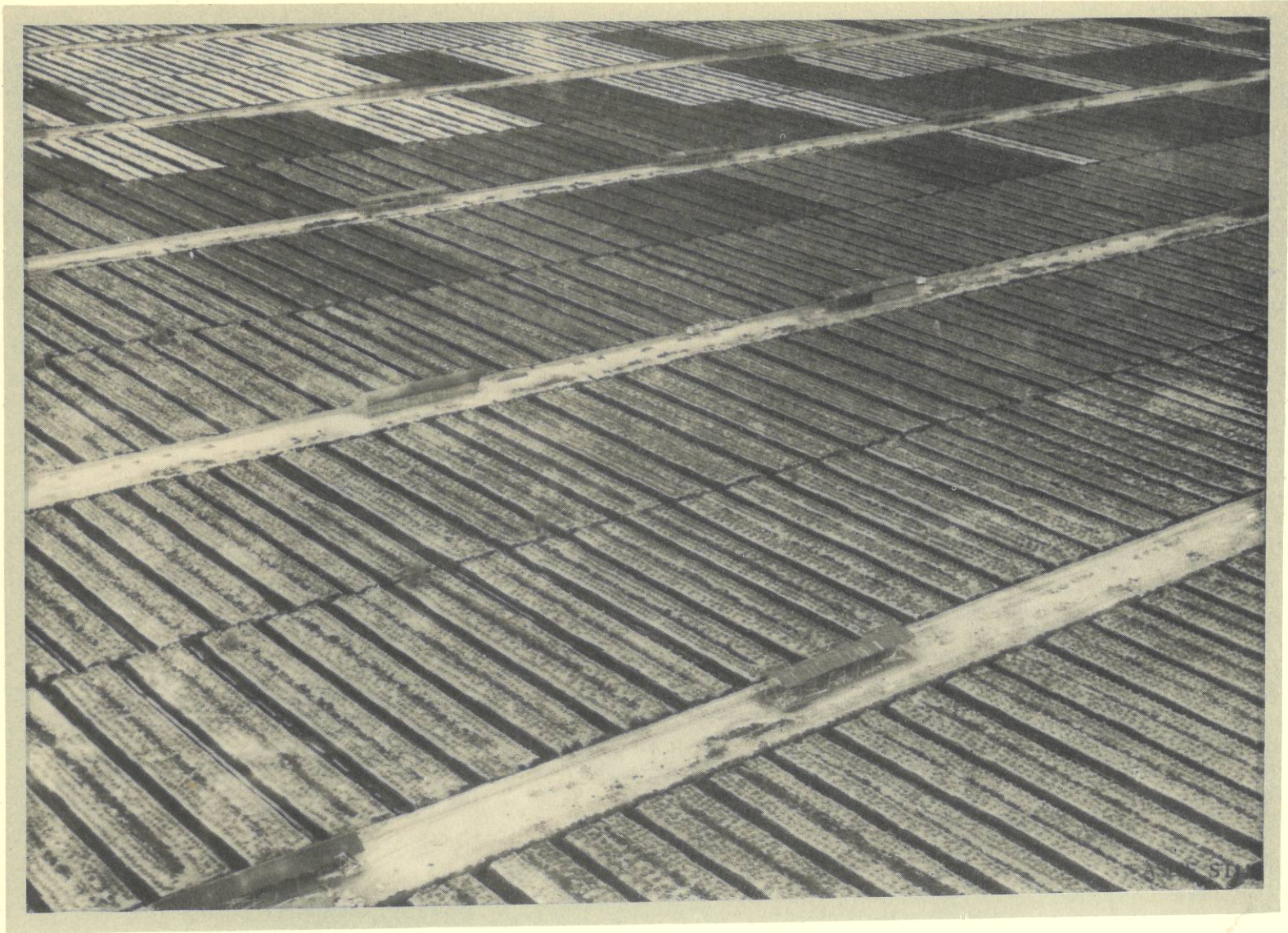
PEAT MOSS CUTTING TRENCHES AND SPREAD FIELDS PEAT MOSS IS CUT BY HAND FROM THE TRENCHES, WEATHERED, FOOTED, HARVESTED AND SUBSEQUENTLY RICKED IN OPEN SIDED DRYING SHEDS ON THE BOG
